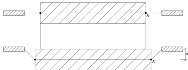
Figure 11 Plan layout of the response of the roof subjected to a transversal displacement.
